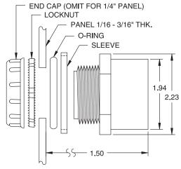
INSTALLATION: INSIDE PANEL SURFACE MUST BE UNIFORM. TIGHTEN LOCKNUT UNTIL SLEEVE BOTTOMS-OUT.
